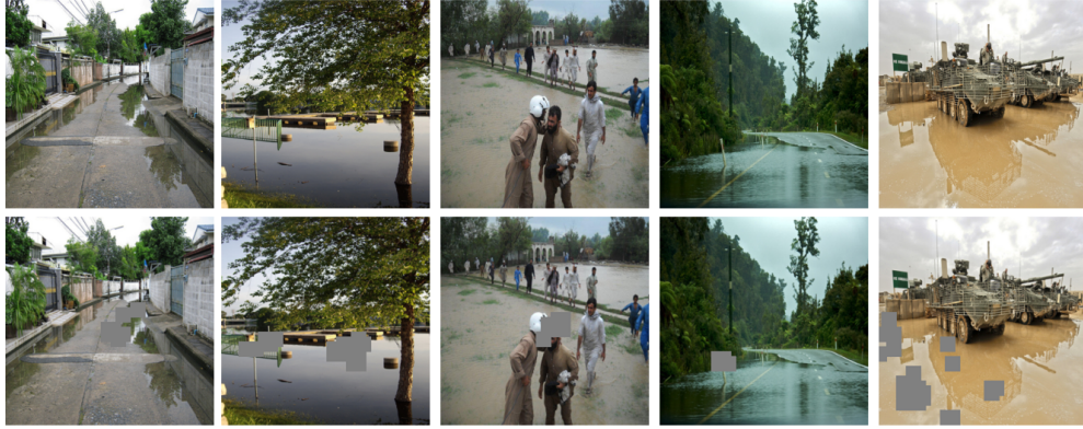
Figure 3: Occlusion sensitivity analysis of five test set examples labeled "flooding". All 19x19 occlusions (separated by a stride of 6) which individually caused the baseline model to erroneously predict "no flooding" are superimposed in the bottom row images.
