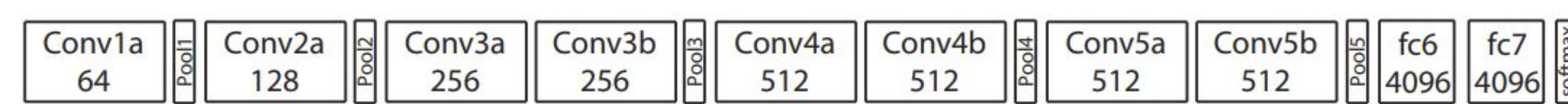
Figure 4: The C3D model depicted above is a shallow 3D CNN model
