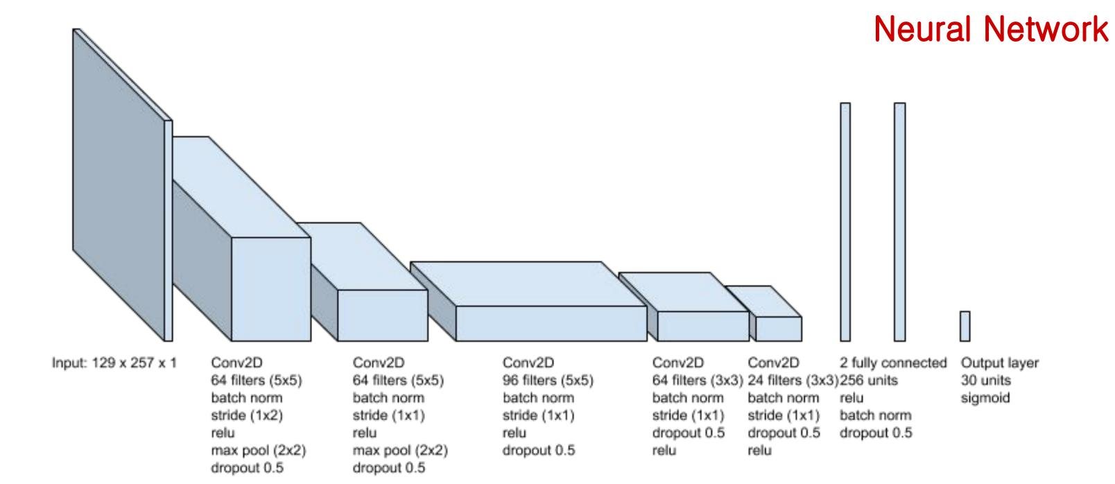
While 1D convolution was initially used for fast feedback on outputs to the model eventually 2D convolution was chosen because it improved more quickly on the loss function.
