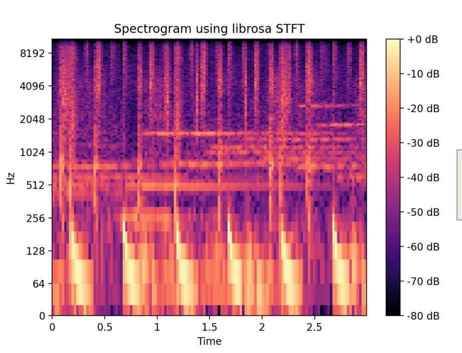
Frequency and amplitude are plotted over the time domain via STFT to produce the image that is fed into the neural network
