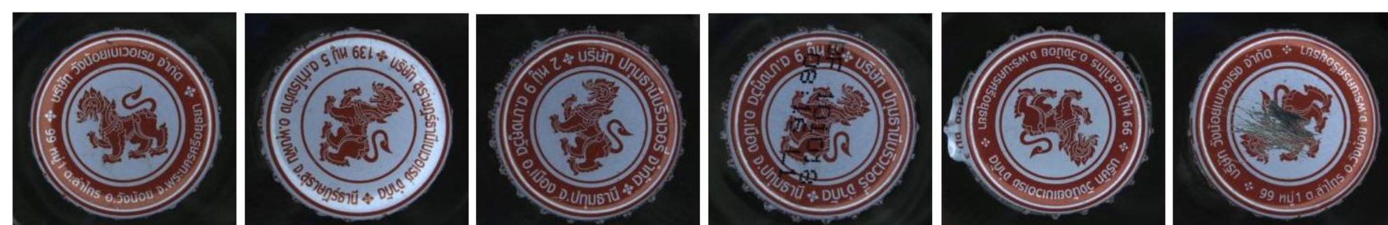
Good Crown y = 0 Color Difference y = 1 Text Difference y = 2 Date Code y = 3 Flare Defects y = 4 Scratch Defects y = 5
