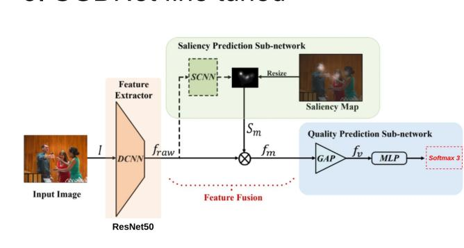
SGDNet is based on ResNet50, and pretrained on IQA Removed last 4 layers, added Softmax(3) Retrained 1,539 parameters
