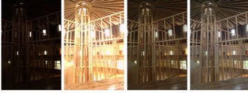
Figure 1: Left to right: an underexposed LDR image, an overexposed LDR image, an image generated with OpenCV's tone-mapping algorithms[10][11] (baseline), and the ground truth.
