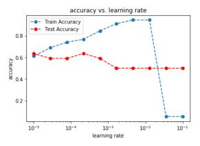
From this plot, we chose a learning rate of 5\*10^-4 and proceeded to iterate on different neuron sizes in the first and second layers of the network. For both of these layers, we iterated from 1-5 neurons, resulting in the following performance visualizations:
