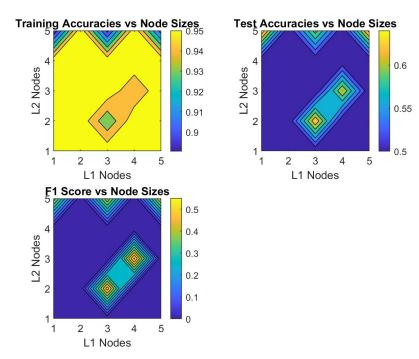
This suggests that a model with 3:2:2 nodes - producing a train accuracy of 94%, a test accuracy of 62% and and F1 score of 0.56 - would perform the best. With this network size, we iterated again through different learning rates.
