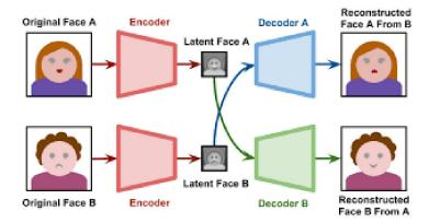
Beside exploring different hyper-parameters, we also introduce GAN algorithm to improve autoenoder's training performance. The structure is simple, we choose training data as real image and autoencoder output image as fake image, use them as intput to train a CNN based discriminator, see below graph for concept.
