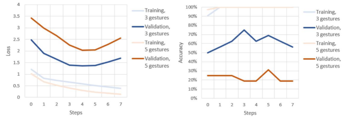
Fig. 5: Performance of the CNN-RNN model when classifying 3 and 5 gestures
