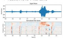
Each input feature vector x<sub>i</sub> had 123 features from a 10ms window of the normalized filter bank
