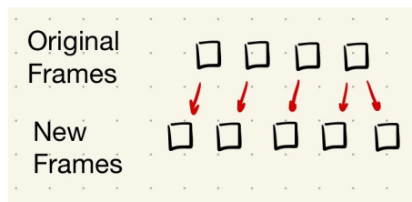
Figure 1: We can see some of the complexities associated with upscaling frame rate above. To keep time, we have to determine which frames must be duplicated and which mustn't be. We do so by decomposing into cycles, analogous to a Fourier Transform.
