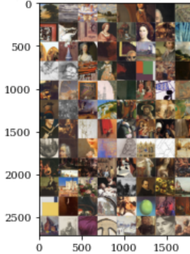
Figure 1: This is a typical set of input for the ResNet at training stage, i.e. an example collection of 96 training images in one mini-batch. Each RGB (3 channels) image is randomly cropped into 224 \times 224 pixels with random flipping applied. The x and y axes labels are the cumulative pixel counts in the two directions for this mini-batch.
