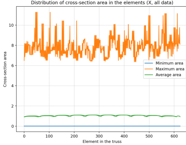
Figure 2: The distribution of the input data shows the high level of dispersion of cross-section area for every element, as well as a similar distribution for every element in the generic truss.
