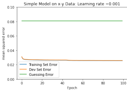
Figure 4: Training and Dev MSE for model M5 over 100 epochs, with ‘guessing error’ shown
