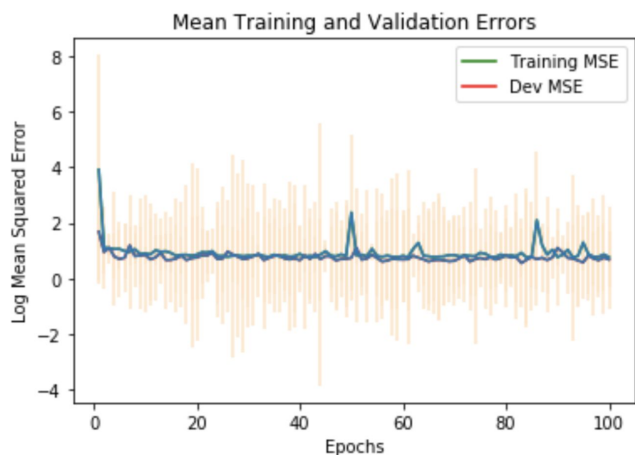
Fig. 8. Mean Log MSE among 5 runs of our best deep learning model plotted with vertical error bars for Training and Dev MSE
