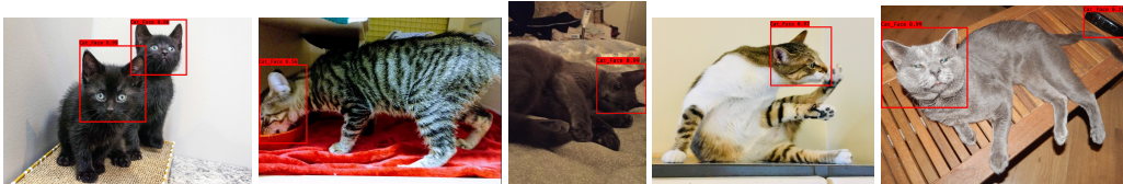
Figure 2: YOLOv3 Cat Face Detection. Note false positive in far right picture: remote control identified as cat with 25% confidence.
