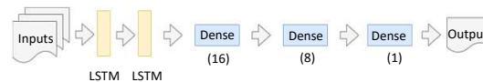
Figure 1: Deep LSTM, two LSTM layers with 64 and 32 hidden units concatenated with three fully connected layers. The first three dense layers used tanh activation and the final dense unit a linear activation.
