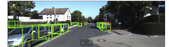
Figure: A sample detection from our trained model. Red/yellow represent ground truth where green presents our model's prediction.
