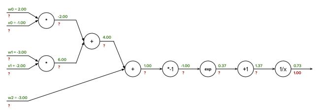
In the graph we've filled out the **forward activations**, on the top of the lines, as well as the upstream gradient (gradient of the loss with respect to our neuron,  $\partial L/\partial \alpha$ ). Use this information to compute the rest of the gradients (labelled with **question marks**) throughout the graph.
