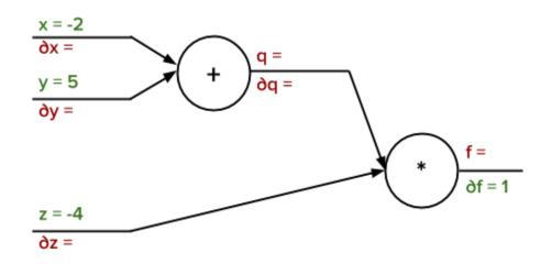
Now let's assume that we are evaluating this function at x = -2, y = 5, and z = -4. In addition let the value of the upstream gradient (gradient of the loss with respect to our function,  $\partial L/\partial f$ ) equal **1**. These are filled out for you in the computation graph.
