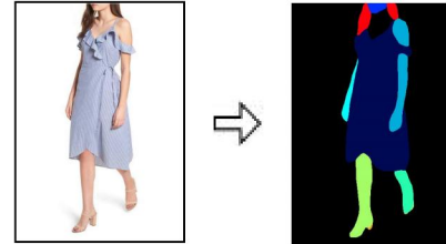
Figure [14]: example of instance segmentation using a catalogue image to generate dress mask
