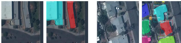
Figure 8. Sample CrowdAI images and predicted masks with the baseline Mask R-CNN model.
