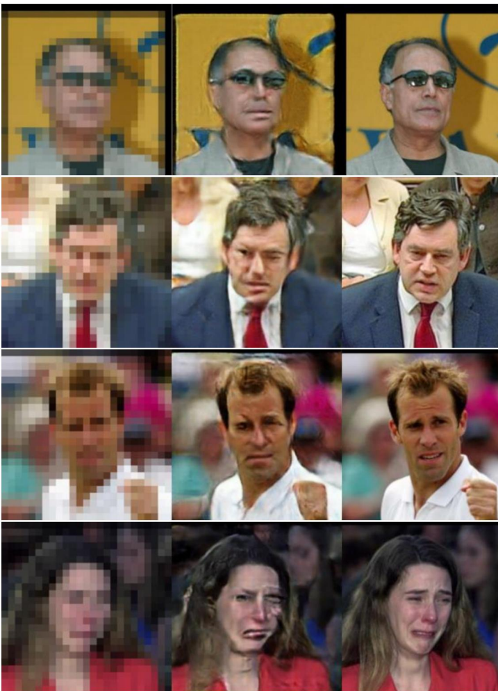
Figure 3. Example results from 25 \times 25 model. From left to right: 25 \times 25 input, 250 \times 250 output, 250 \times 250 target.
