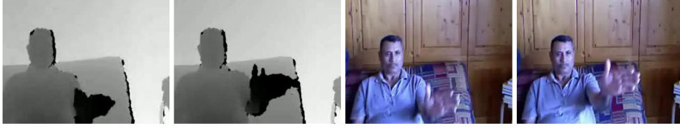
Figure 1: Kinect RGB-D (left) and RGB (right) video frames depicting an actor performing a handshake gesture, occurring adjacently at a video sampled at 10 fps.
