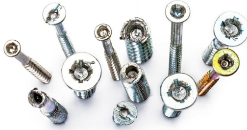
Figure 1: Example of broken screws from applying pressure using screw bit with inappropriate fit.
