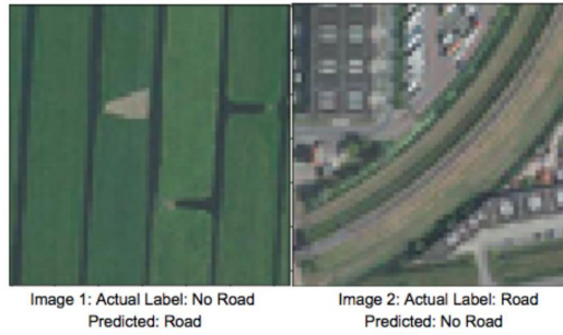
Figure 5. Error Analysis for Pixel-Level Road Detection
