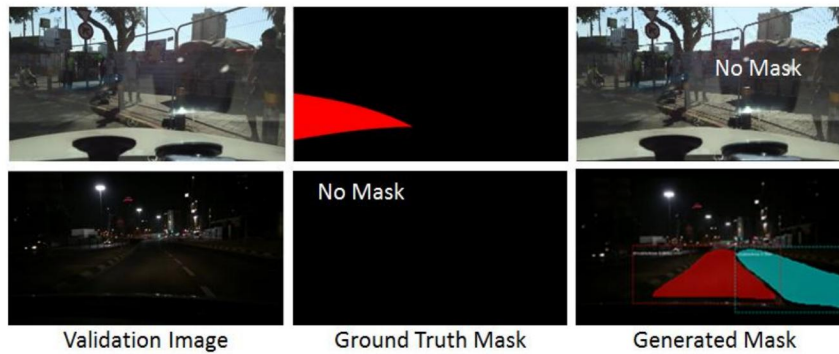
Figure 4: For the final training run (experiment 8 in table 1)- Two example images, corresponding ground truth mask and generated mask. For both the cases estimated \text{IoU} = 0 . Bigger size images and more result visualization can be found in the github repo.
