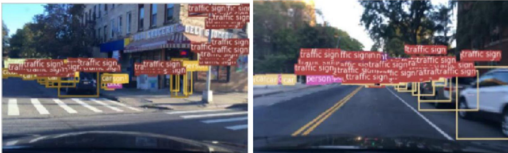
Figure 5: Baseline model has high false positive rate on smaller objects
