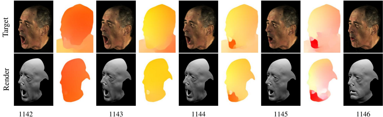
Figure 2. We use optical flow to infill frames where the face detector fails. Starting from frame 1142, the optimization moves the head to match the optical flow of the synthetic render to the optical flow of the captured image. After solving for frame 1145, we perform another round of optimization except that we start from frame 1146 instead; this way, each frame will capture optical flow information from both anchor frames. Using optical flow allows the mouth to stay open longer ( e.g. in frame 1144) than what one would obtain using simple interpolation.
