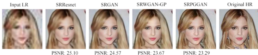
Figure 5: Input LR 32x32, SRResnet 4x output, SRGAN 4x output, SRWGAN-GP 4x output, SRPGGAN 4x output, Original HR 128x128
