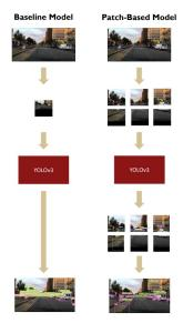
The two models used the same standard YOLOv3 network architecture. The architecture's loss function is provided
