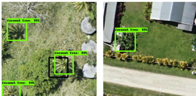
Images 3 and 4 On the left: An incorrectly classified coconut tree shadow. On the right: Banana trees that the classifier believes are coconut trees.
