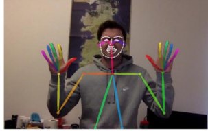
Figure 1, sample image from a sign video for “awful” with the OpenPose keypoints rendered on top of it
