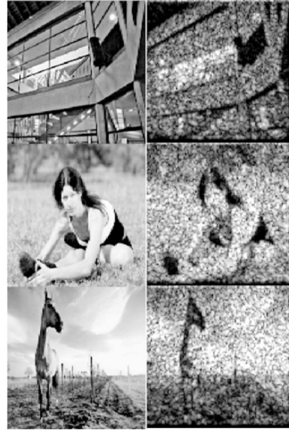
Fig. 3: Example training data, the left column shows the original image before simulation, this will be used as a label. The right column shows the simulated speckled image, this will be used as the input
