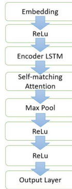
Figure 6: The final modified BCN architecture after overcoming memory and overfitting issues.
