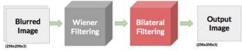
Figure 4. Architecture of the network we were comparing to. The network is shown here with bilateral filtering added as the last layer.
