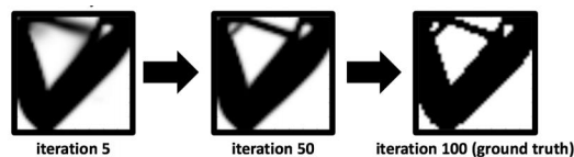
Figure 3: Each of the 10,000 datapoints contains iterations 1 through 100 from the topology optimization; iterations 5, 50, and 100 are shown here.
