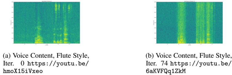
Figure 4: The following spectrograms show the generated audio after the first iteration and 75th iteration of training with vocal audio as content and a flute tone as the style. We find that the vocal audio using the Gram matrix loss with style layers at the first ReLU activation units preserves the content audio temporally (we can still understand what is being said) but the original frequencies are blurred to other frequencies.
