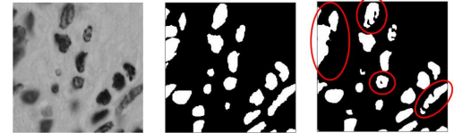
Figure 4: Sample Error. Left, raw microscope image. Middle, predicted mask. Right, ground-truth mask label. Errors include conjoined masks as well as masks that leak information as a result of imaging quality; this includes finger-like projections, "holes" in masks, and split masks. Example errors circled in red.
